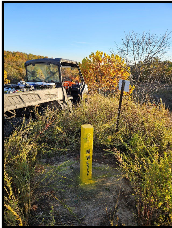
Photograph 6: View of re-painted and re-labeled stickup at MW-577.
