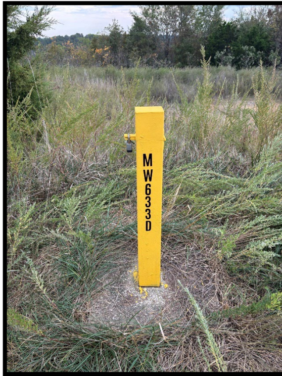
Photograph 7: View of re-painted and re-labeled stickup at MW-633D.
