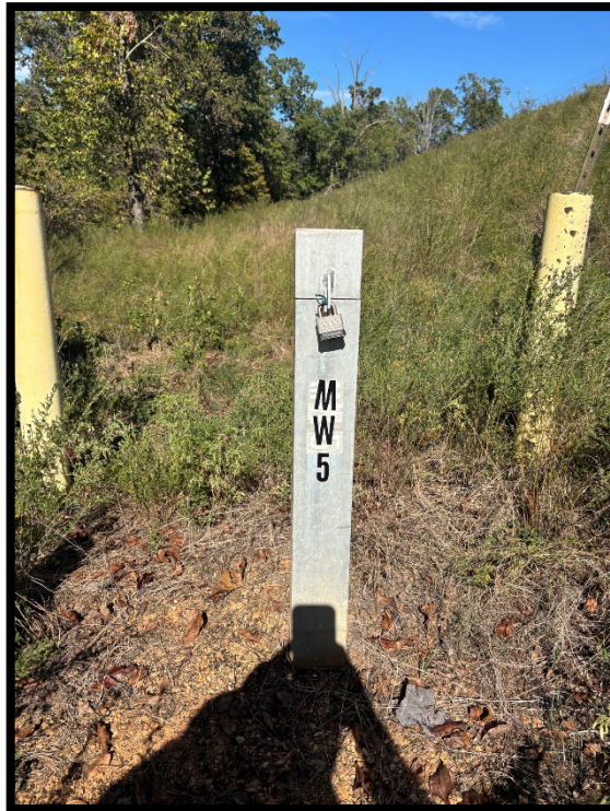
Photograph 4: View of re-labeled stickup at MW-5.
